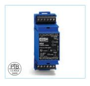
If the nominal response temperature in PTC thermistors reaches a set limit the built-in relay disconnects the motor. The fault is indicated by a light emitting diode. Restarting via pressing the "Reset" button or an external switch. Casing made of polymer, suitable for fuse board installation on support rail according to DIN EN 60715.
